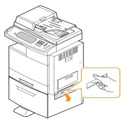
2 Open the inner cover of the high capacity feeder.
